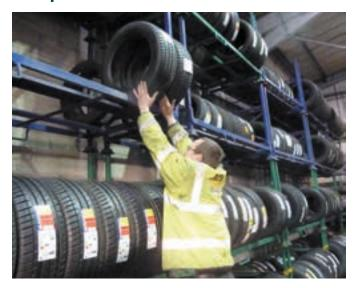
While storing tyres in racking is common, this may not reduce all potential handling risks. It is natural to put frequently handled tyres on the lower racks and those less frequently handled high up. But, unless other aids are used, this will create unnecessary risks, including:
